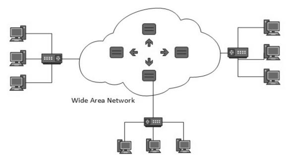
WAN may use advanced technologies such as Asynchronous Transfer Mode (ATM), Frame Relay, and Synchronous Optical Network (SONET). WAN may be managed by multiple administration.
