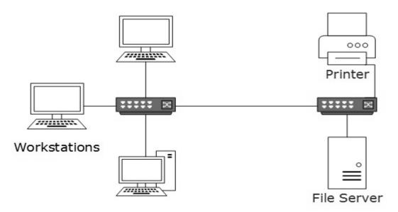
LANs are composed of inexpensive networking and routing equipment. It may contains local servers serving file storage and other locally shared applications. It mostly operates on private IP addresses and does not involve heavy routing. LAN works under its own local domain and controlled centrally.
